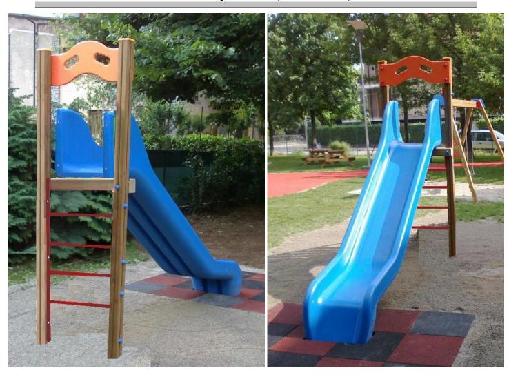
Certified according to European Standard EN 1176. Realized in painted aluminum 3mm thick The whole structure is constituted by poles of sec. cm.  $9 \times 9$  with rounded corners. Ladder realized in galvanized and painted steel. Entrance slide panel in polyethylene. Polyethylene slide manufactured from 6 mm thick rotationally moulded high density, UV Stable and with a characteristic final wave.
